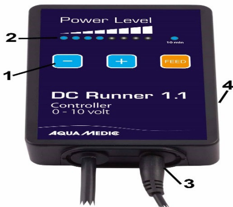
Fig. 3: DC Runner Controller 1.1
